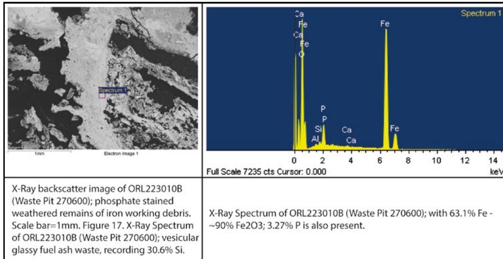
X-Ray backscatter image of ORL223010B (Waste Pit 270600); phosphate stained weathered remains of iron working debris. Scale bar=1mm. Figure 17. X-Ray Spectrum of ORL223010B (Waste Pit 270600); vesicular glassy fuel ash waste, recording 30.6% Si.
