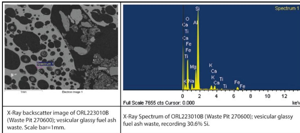
X-Ray backscatter image of ORL223010B (Waste Pit 270600); vesicular glassy fuel ash waste. Scale bar=1mm.
