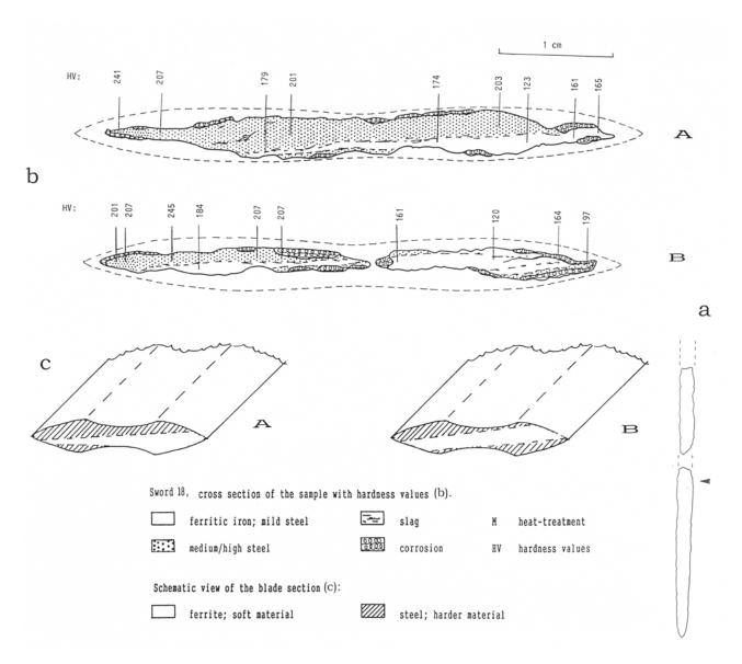
Figure 6.19a. Sword 18. Cross-section of the sample with hardness measures (b), schematic view of the blade section (c) and outline of sword with section marked (a).
