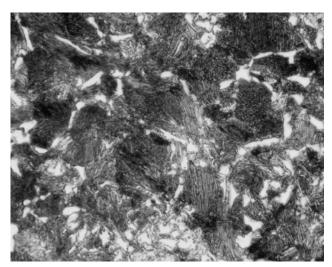
*Figure 6.21f.* Sword 20. The left edge consists of lamellar pearlite with medium to high carbon content. (500x).
