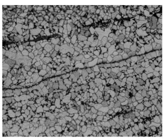
**Figure 6.21e.** Sword 20. Ferrite layers separated by lines of pearlite and slag and hammer scale bands running across the entire central part. (100x).
