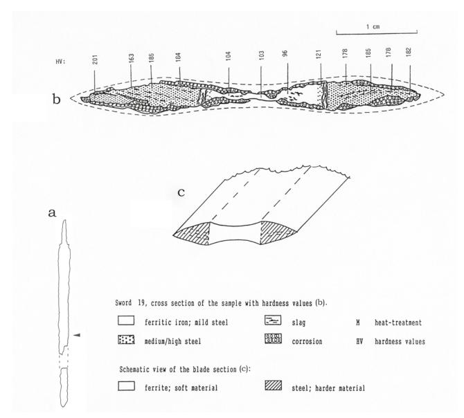
Figure 6.20a. Sword 19. Cross-section of the sample with hardness measures (b), schematic view of the blade section (c) and outline of sword with section marked (a).
