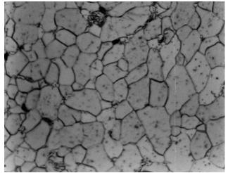
*Figure 6.19e.* Sword 18. A ferritic layer runs obliquely in an edge-to-edge direction. (500x).
