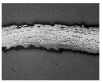
**Figure 6.21c.** Sword 20. Most of the central part consists of layers of ferrite separated by numerous lines of pearlite and bands of slag and hammer scale running parallel from edge to edge. Etched in nital. (20x).
