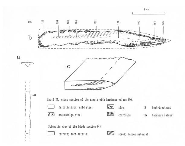
Figure 6.22a. Sword 21. Cross-section of the sample with hardness measures (b), schematic view of the blade section (c) and outline of sword with section marked (a).
