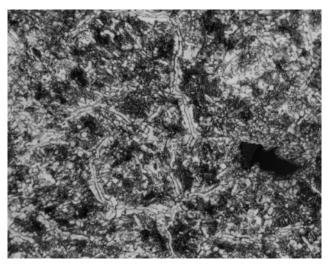
**Figure 6.21g.** Sword 20. The right edge consists of medium to high carbon steel with cementite in the prior austenite grain boundaries. (500x).
