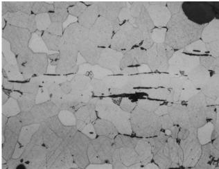
Figure 6.14e. Sword 13. The core is mostly ferritic. (200x).
