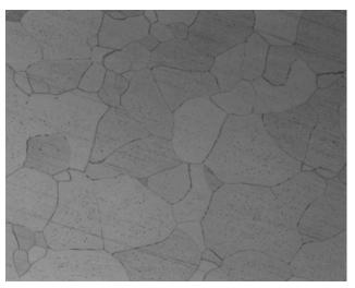
Figure 6.13c. Sword 12. The entire sample consists mostly of pure ferrite. (200x).
