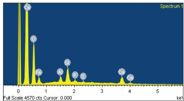
**Figure 27.14.** Fryasletta: As Fig. 11, X-ray spectrum of iron-void infills (EDS analysis); iron is dominant (43.2% Fe), with 1.73% P, 6.33% Ca, and 0.59% S (relict root?). Local silts contain 5.54% Fe and 0.24% P.
