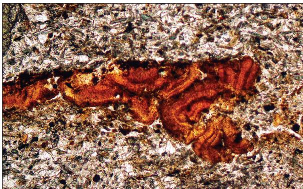
**Figure 27.13.** Fryasletta: Photomicrograph of M63A, layer 9; minerogenic alluvial silts, with reddish brown secondary iron-void infills ('ferrihydrite?'). PPL, frame width is 0.90 mm.
