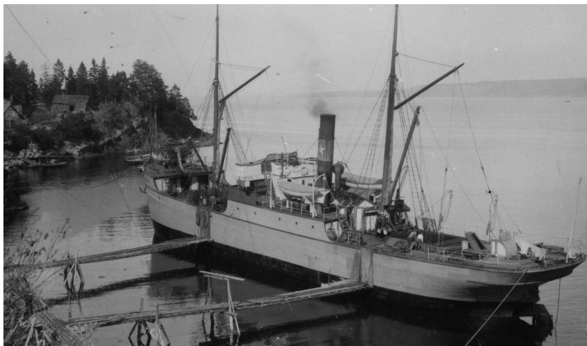
Picture 5-6. Wooden steamship loading ice using steam winches and derricks.
